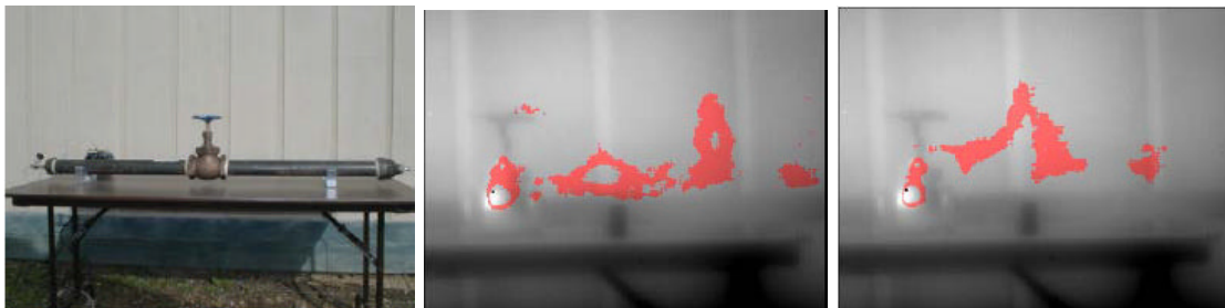
Fig. 8. IMSS Images of Valve Leaking Methane
