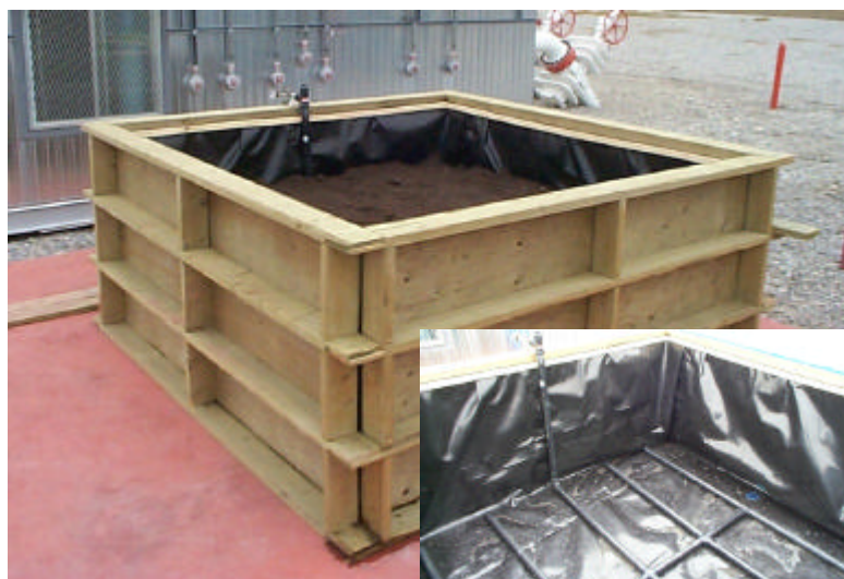
Figure 3: Field biofilter and its gas distribution pipe network
